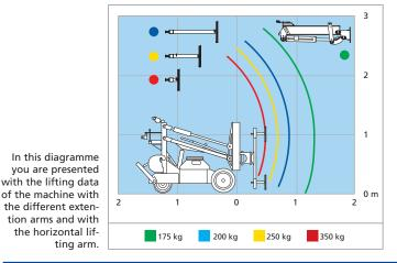
With the horizontal lifting arm as an optional extra you are able to pick up loads from ground level and mount it up to 3,2 meters.
