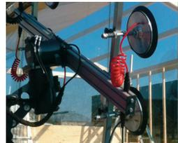
A two-circuit vacuum system ensures that the suction discs always have 400% overcapacity. A visual - and an acoustic alarm ensure that the machine is not operated until the system has reached optimum suction power. This makes the vacuum system one of the safest systems in the world.
